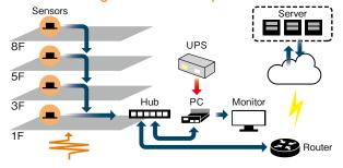
This system uses data from multiple vibration-detecting sensors to calculate and determine the degree of damage. After installation, this system collects and stores all information from subsequent seismic events, automatically calculating the cumulative damage to the building structure. Even for an earthquake with multiple, strong foreshocks and shocks, the system can make a determination of safety level of the earthquake based on foreshocks.
