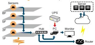
This system uses data from multiple vibration-detecting sensors to calculate and determine the degree of damage. After installation, this system collects and stores all information from subsequent seismic events, automatically calculating the cumulative damage to the building structure. Even for an earthquake with multiple, strong foreshocks and shocks, the system can make a determination of safety level of the earthquake based on foreshocks.
